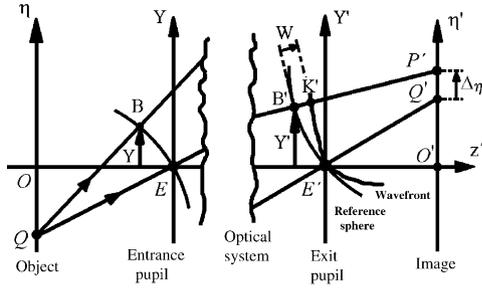
**Fig. 1.** Coordinates in the object, image and pupils planes.  $Q$  and  $Q'$  are an object point and its ideal image point while  $E$  and  $E'$  are points at the entrance and exit pupils centres; respectively,  $QEE'Q'$  is the principal ray and  $QBB'Q'$  is an arbitrary ray.
